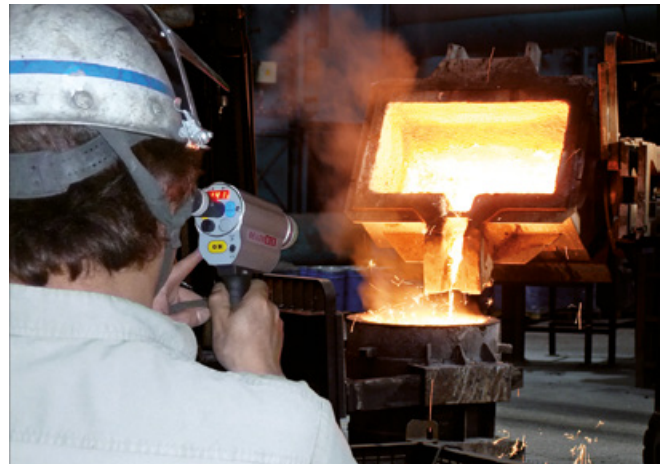
Fig. 7 A portable panorama pyrometer measures the temperature during the pouring process.
