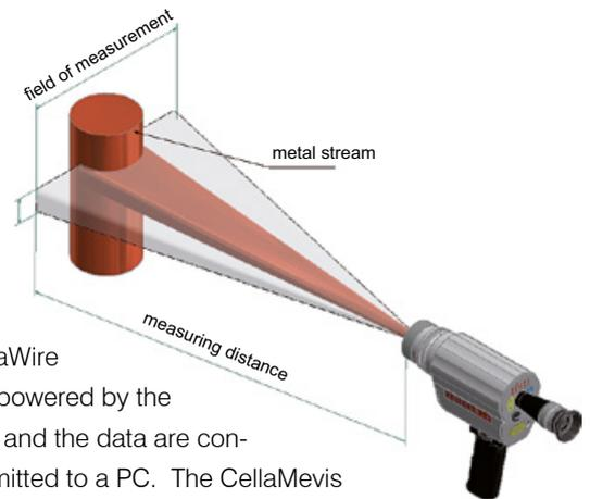
CellaCast PT 143 comprises different models for temperatures ranging from 600 °C to 3000 °C. Four interchangeable lenses are available for different target distances and sizes for applications involving wire diameters from 2mm upwards. Additionally, the optical resolution can be enlarged by mounting supplementary lenses to the pyrometer to capture target spots as small as 0.3 mm.
