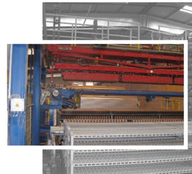
Dryer car loading station
