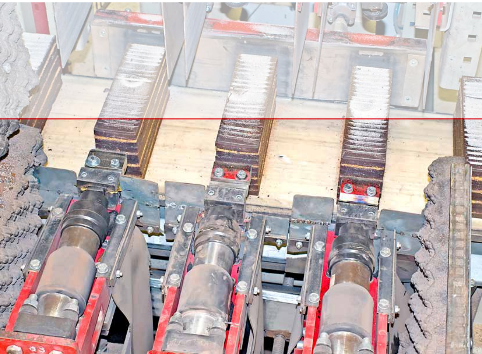
Splitting/separating of facing strip stacks
