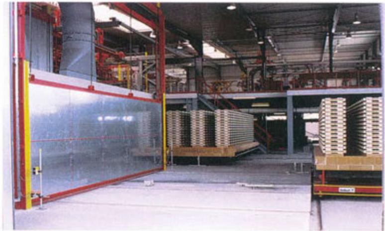
Ofenausfahrt, Ofenwagen-Schiebebühne und 2-Stock-Betrieb Kiln exit, kiln car transfer car and two-storey operation
