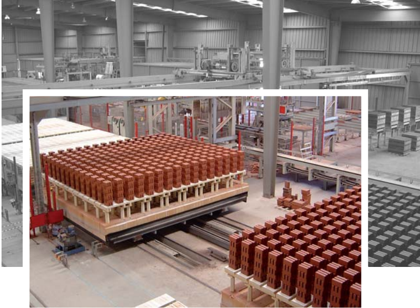
Overview tunnel kiln car unloading
