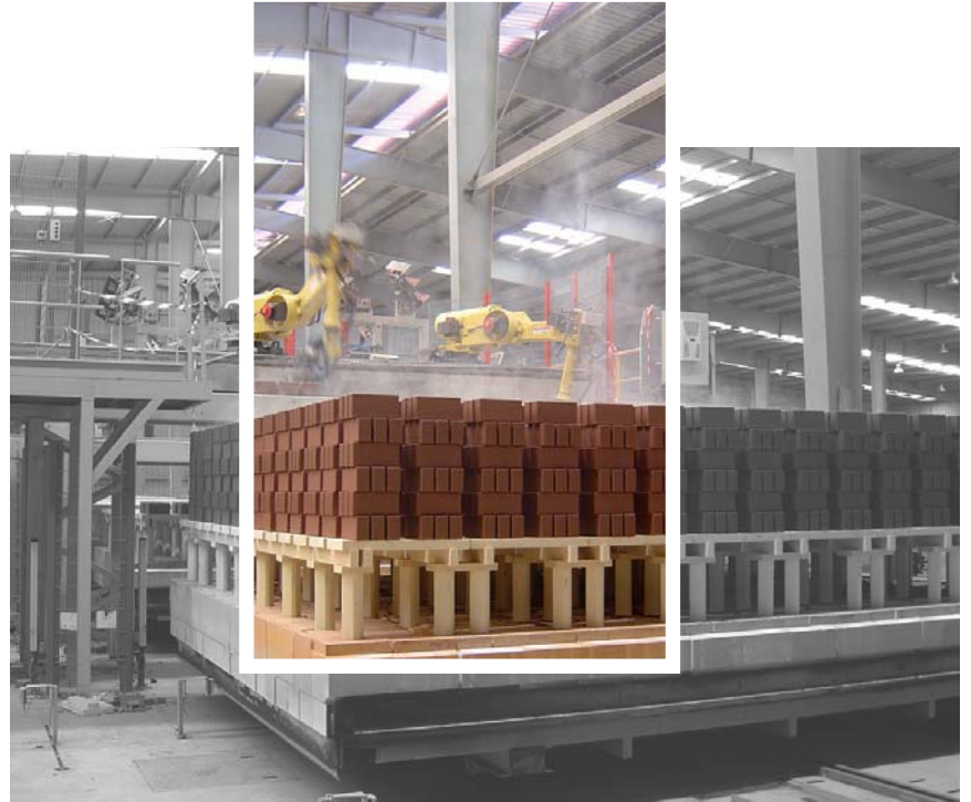
Loaded tunnel kiln car
