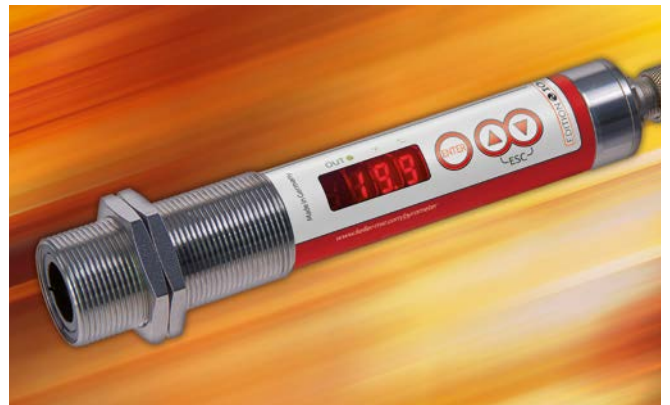
Pyrometers of the CellaTemp PK 41/42 series with their spectral sensitivity of 4.6 – 4.9 \mu\text{m} measure temperatures just below the glass surface.
