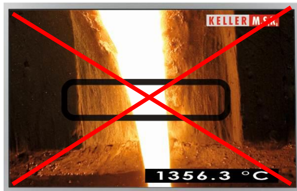
Incorrect aiming captures the target and the hot background
