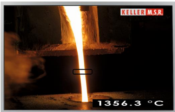
Correct aiming captures the free flowing molten metal stream
