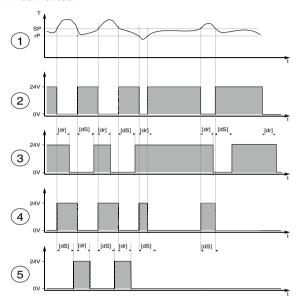
T = temperature P = P = lower limit value t = time P = P = switch on delay P = P = switch off delay
