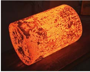
Fig. 4 Scale particles on the block surface often lead to irritations with the contactless measurement of the surface temperature.
