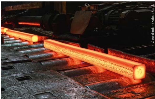
Fig. 2 Scale and oxide significantly change the radiation properties.
