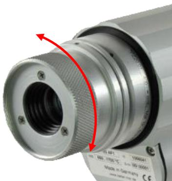
The pyrometer is equipped with focusable optics. Turn the lens until the target object **and** the target marker (distinctly marked in the viewfinder) **both** appear in sharp focus simultaneously
