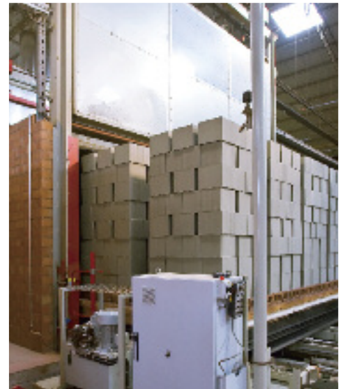
Kiln entrance with sluice which is arranged upstream.
