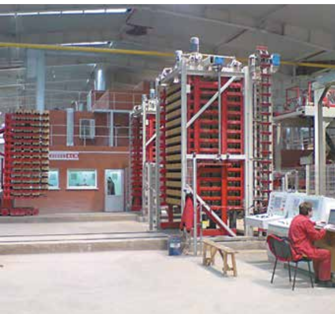
Trocknerwagen-Beladung Dryer car loading
