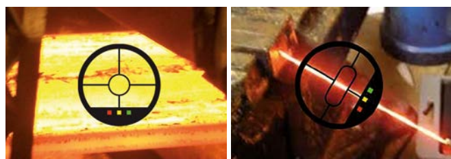
Patented traffic light function in the view finder of the CellaPort PT
