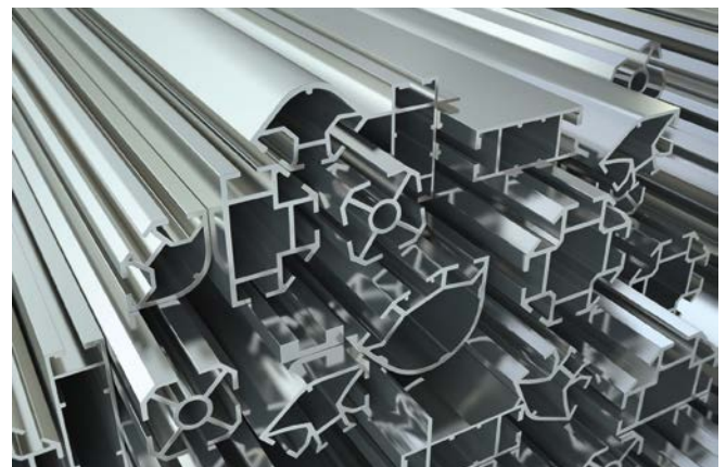
Fig. 3 The profile of the aluminium can influence the infrared temperature measurement.
