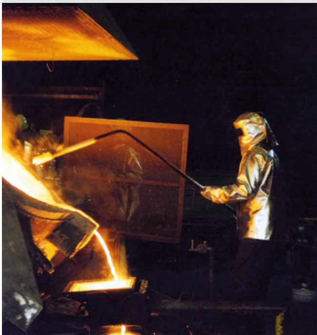
Fig. 1 Conventional temperature measurement of liquid metal using an immersion probe
