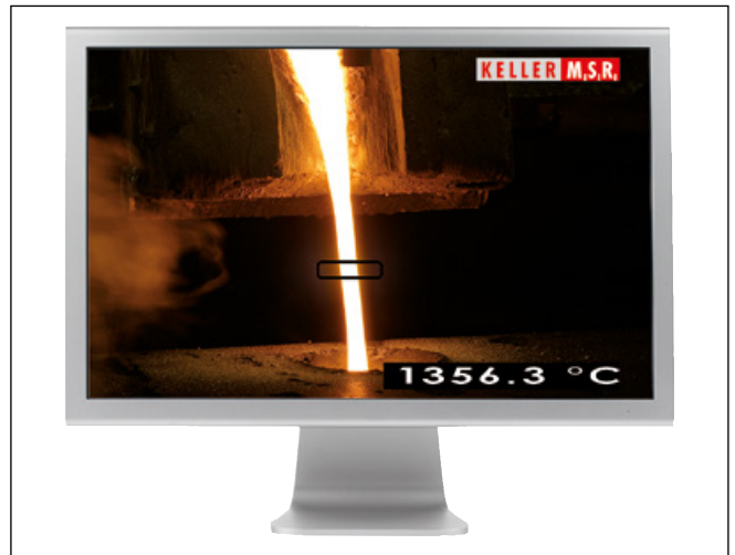
Fig. 8 Video image shows targeted measurement area and superimposed temperature reading
