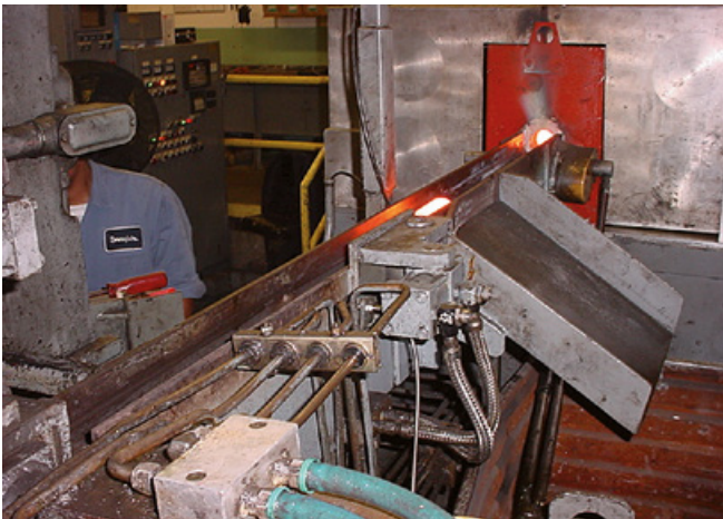
Fig. 1 Billet rejection based on temperature
