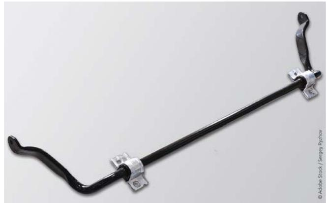
**Fig. 1** Chassis stabilizer of an automobile
