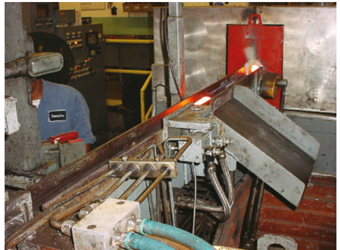
Fig. 9 Gate to discard billets with too high or too low temperatures.
