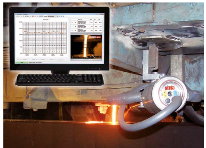
Fig. 4 Measuring point at the automatic casting machine and monitor for displaying the casting temperature and the video image.
