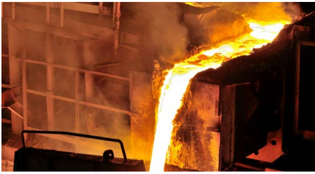
Fig. 3 Measuring point casting channel with slag and oxides on the flowing melt.
