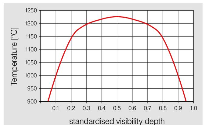
**Fig. 4** Temperature profile inside the combustion chamber
