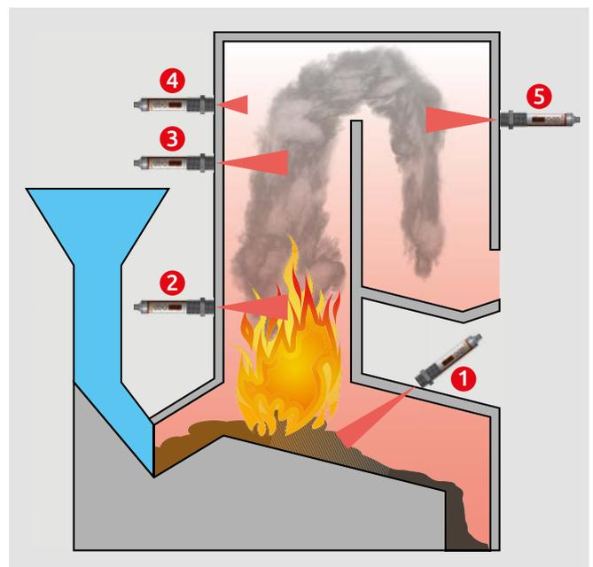
**Fig. 1** Principle representation of the different measuring locations in a combustion chamber
