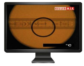
Video image optained by the pyrometer CellaTemp PA with video camera through a sighting tube inside a dark furnace
