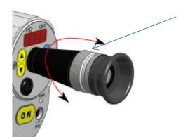
The pyrometer offers diopter compensation to adjust the sighting device to the user's vision. Turn the ring until you see a sharp image of the target spot indication in the viewfinder.
