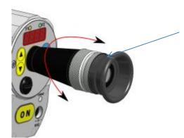
Instruments with a measuring range of > 2000 °C are equipped with a polarisation filter to control brightness and protect the user's eye.
