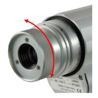
The pyrometer is equipped with focusable optics. Turn the lens until the target object **and** the target marker (distinctly marked in the viewfinder) **both** appear in sharp focus simultaneously
