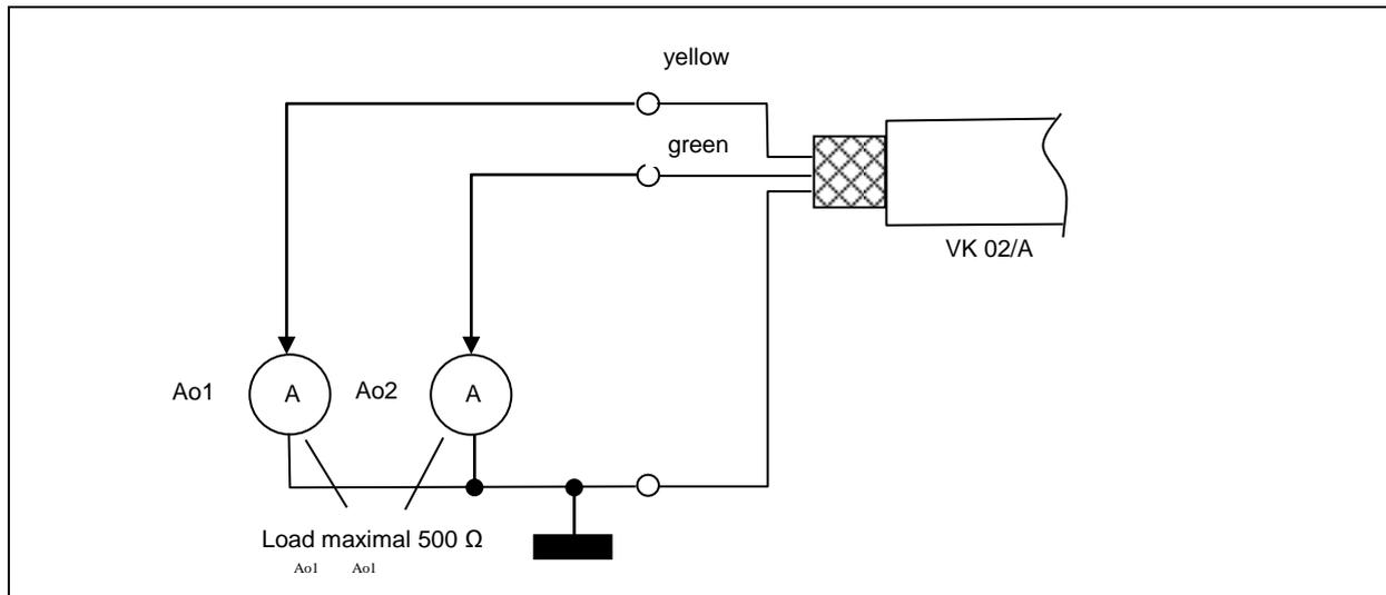
For all pyrometers of the PA Series the current outputs are short-circuit-proof and share one ground connection via pin 8 of the connector. Each current output can be individually scaled and can be set either at the display or via interface.
