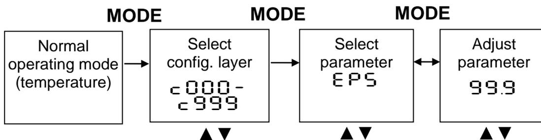
1. Press the MODE button while in normal operating mode to switch to "configuration layer" mode.
