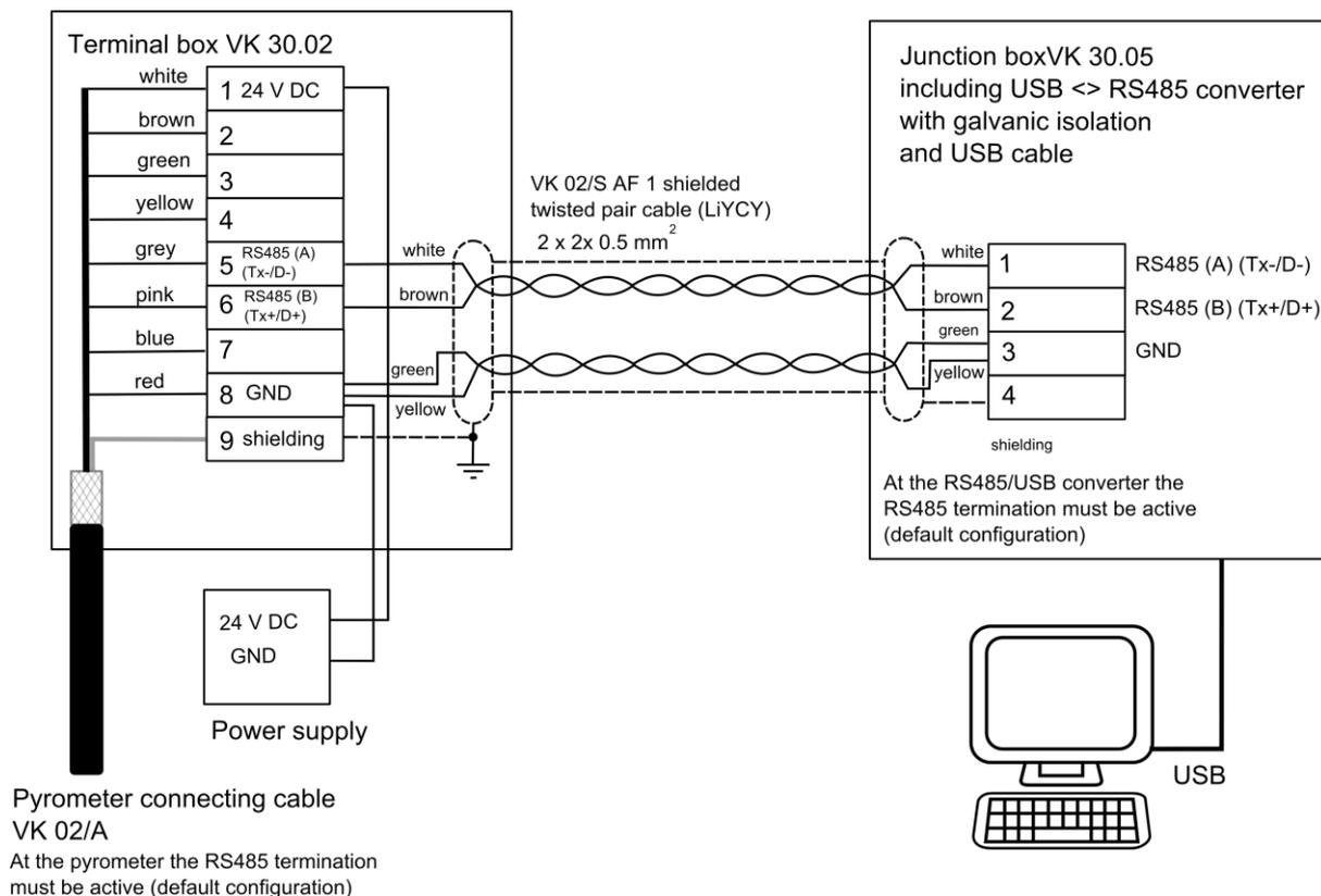
Moreover, use a converter with galvanic isolation (e.g. W&T 38211) to avoid problems with ground loops.
