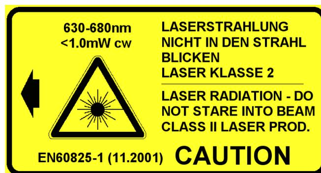
Fig. 5.2 Laser warning label affixed to the pyrometer
