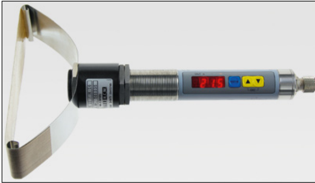
Fig. 6 Bow with a Teflon tape to measure shiny rollers.
