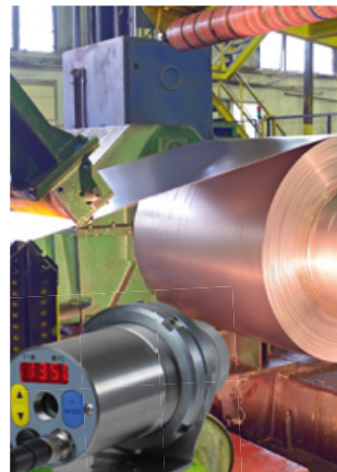
Fig. 8 Continuous-wave sensor pyrometers to measure temperatures from 75 °C upwards.
