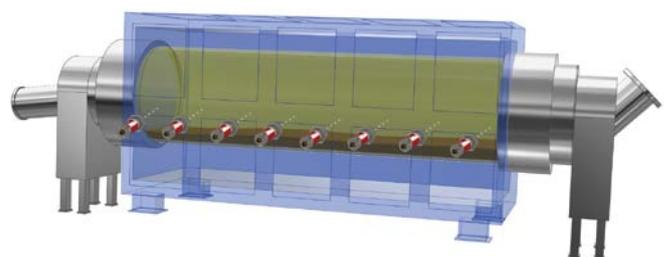
**Fig. 2** Indirectly heated rotary kiln with one measuring system per burner zone
