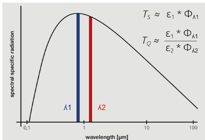
**Fig. 1** Spectral pyrometers measure the radiation ( $T_S$ ) at one wavelength, whereas two-colour pyrometers determine the temperature from the ratio of the radiance of two wavelength ranges ( $T_Q$ )
