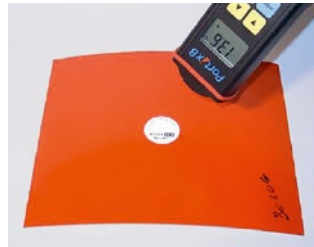
Fig. 2 Determine emissivity by comparison measurement on emission adhesive tape with defined emissivity.
