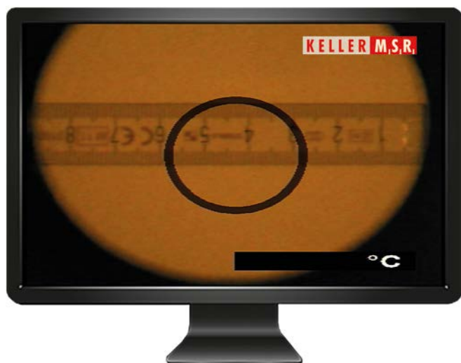
Video image obtained by the pyrometer CellaTemp PA with video camera through a sighting tube inside a dark furnace
