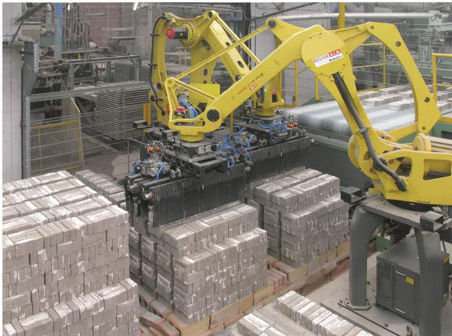
*Two 4-axis palletizing robots with pneumatic spacing grippers for setting soft mud bricks on kiln cars
