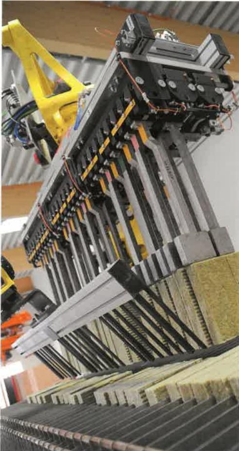
*Sting gripper to pick up the mineral wool cuttings
