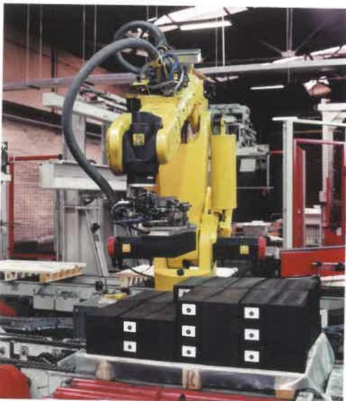
*Refractory material handling with suction gripper
