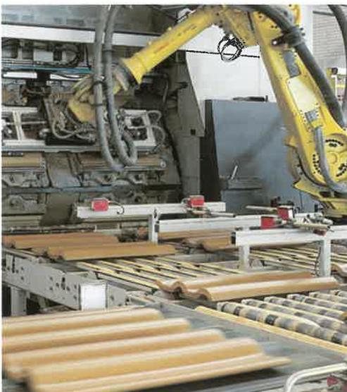
Also roof tiles are exposed to the risk to be deformed during the loading and unloading of the roof tiles press due to their preparation water content and their form and size. Therefore, the robots and grippers for loading and unloading of roof tile presses must be designed in a very sensitive way.
