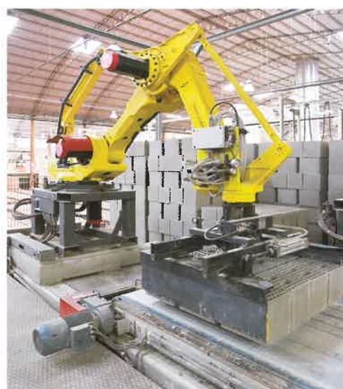
*4-axis palletizing robot with pneumatic gripper
