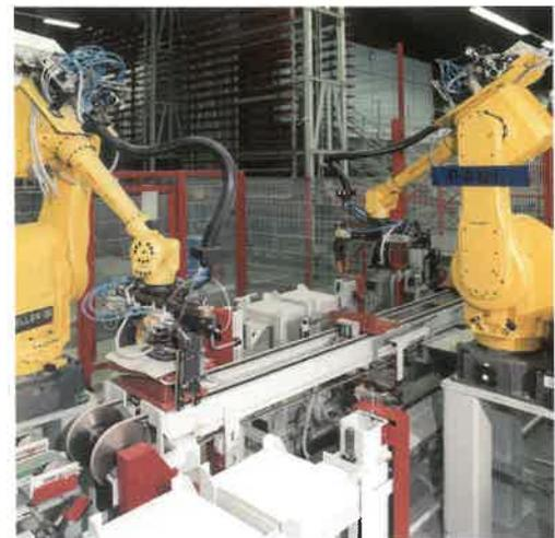
Two 6-axis articulated robots with combined gripper and suction device form packs with accessory tiles with an intermediate paper layer
