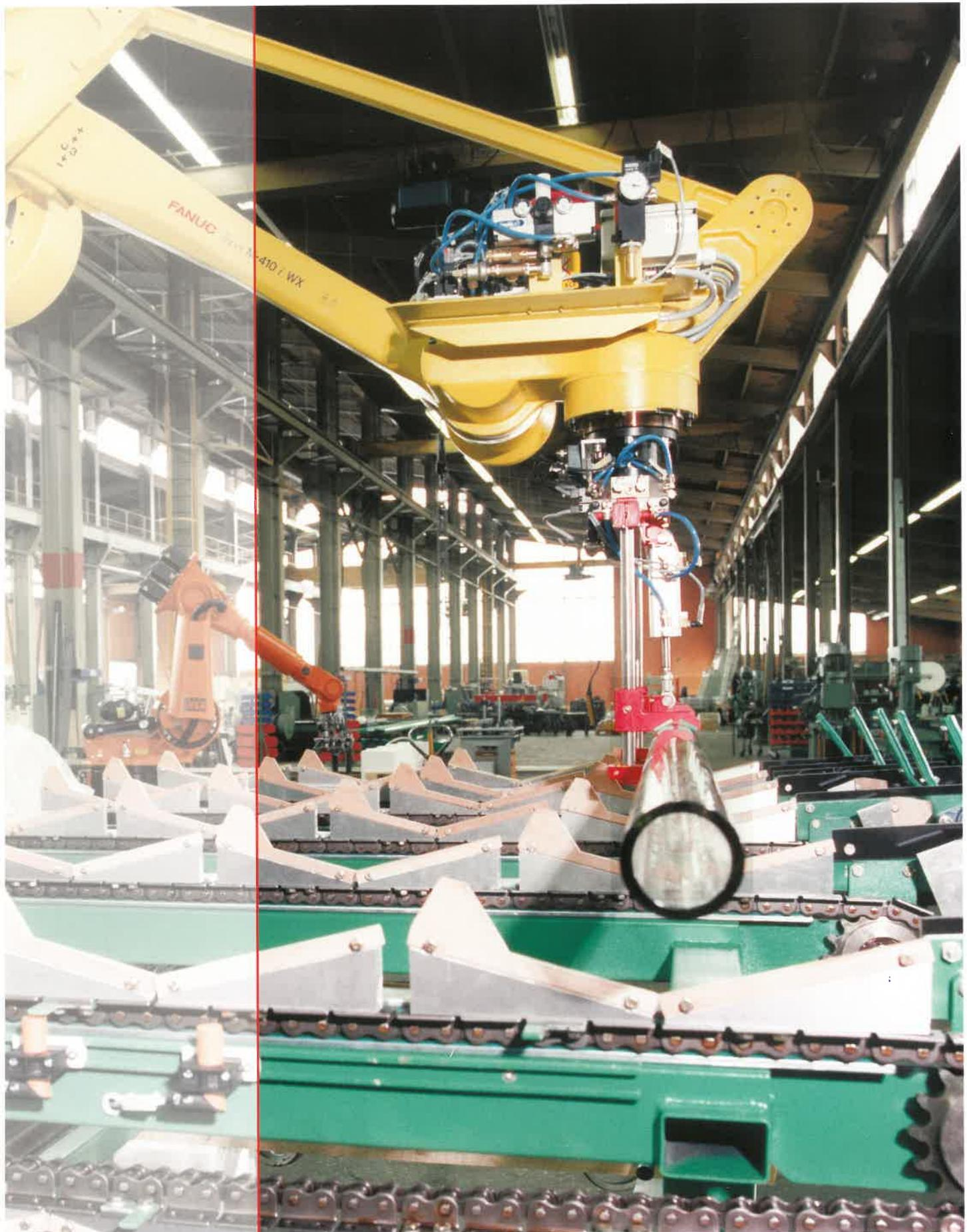
Handling of glass tubes with special grippers during test run at KELLER in Ibbenbüren-Laggenbeck
