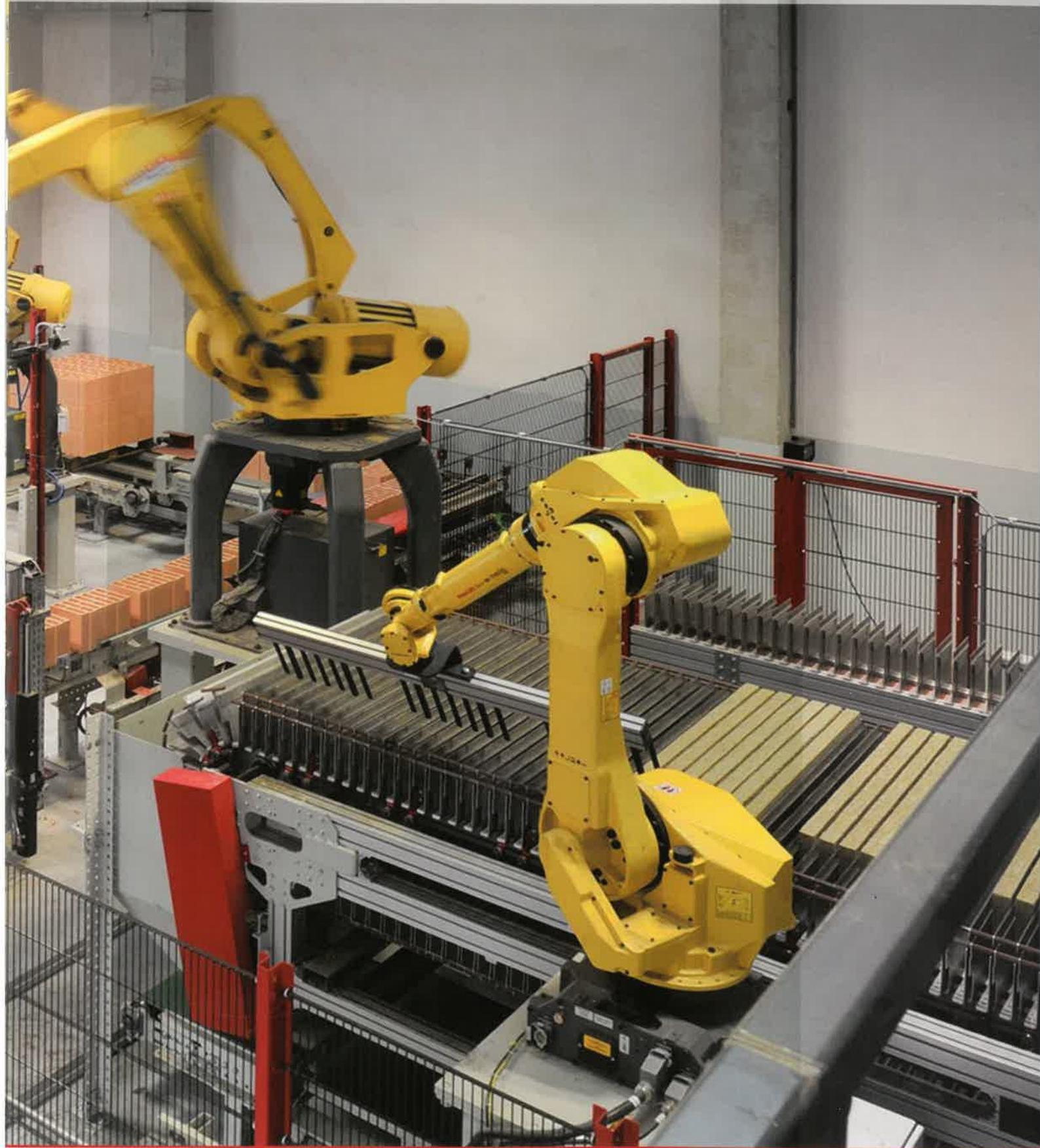
For the transport to the customer the robots stack the finished facing bricks, common bricks and pavers directly on pallets which are then welded or strapped with belt. In case of roof tiles, roof tile accessories, floor tiles and facing strips, the finished products are first combined in packs by 6-axis articulated robots, which are then optionally welded, strapped with belt or packed in boxes.
