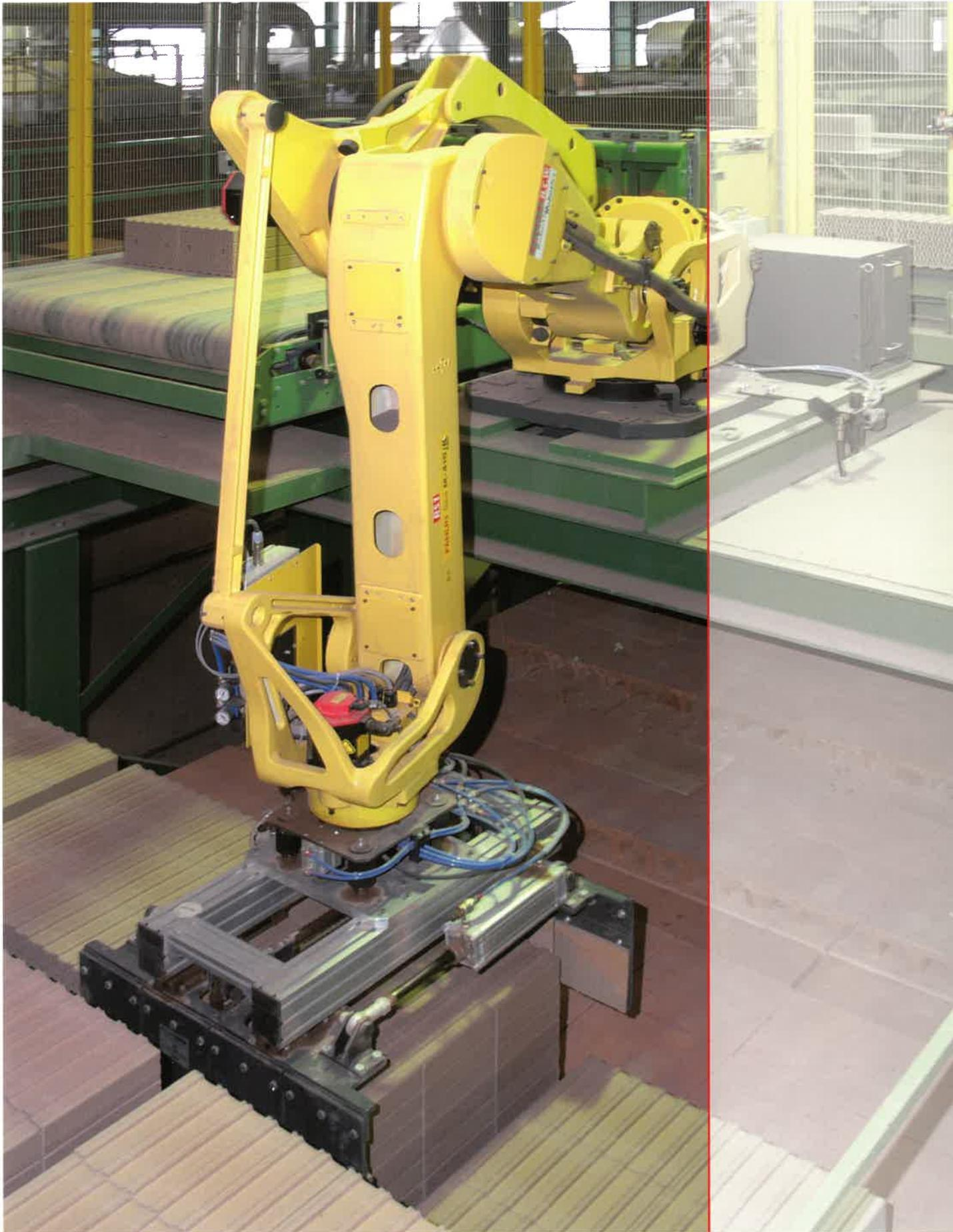
4-axis palletizing robot with pneumatic gripper for setting common bricks on kiln cars
