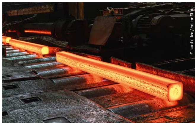
Scale and oxide significantly change the radiation properties
